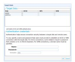
Figure 37. The "Target Mode" window is used to allow computers and third party software to remotely connect via iSCSI to disks connected to Ditto.
